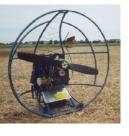
about as much noise as a lawnmower and when more than a few hundred feet away, most people do not find it objectionable. The noisiest type of motor, the direct drive, is louder but few of those are utilized owing to the reduced thrust and higher noise.
